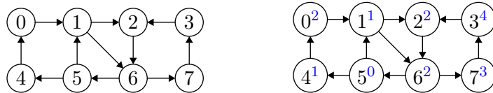
Figure 13.1: Breadth-first search of a graph.
